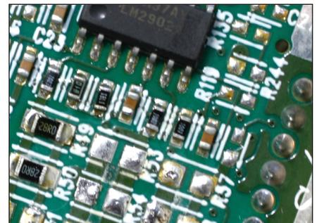
Figure 4 — The board should look like this. Two 0603 size resistors have been removed, and the cleaned board is ready to receive two new resistors.
