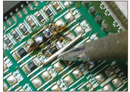
Figure 1 — A small piece of bus wire is used to transfer heat to both sides of the component at the same time.
