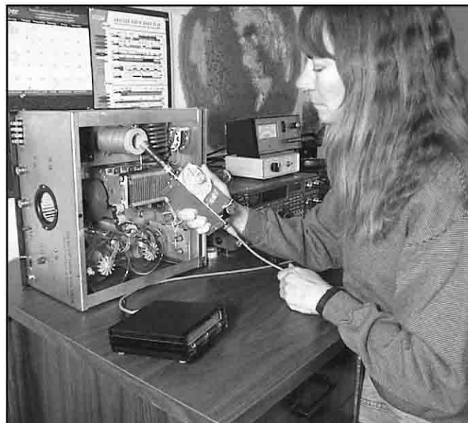
Figure 6—N3SU grid-dipping her linear amplifier's tank coil. Note that the high-voltage power supply is not only off but is disconnected from the amplifier.
