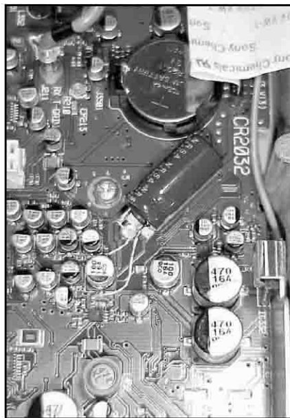
Figure 1—Add a capacitor to cure audio rumble in ICOM IC-765PRO and PROII.
