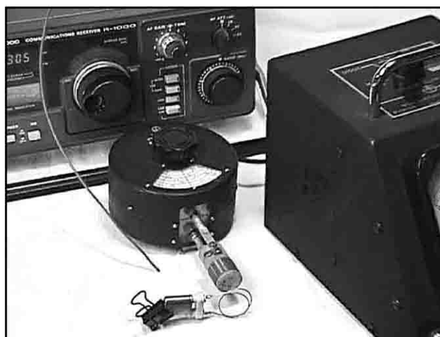
Figure 6—A calibrated receiver is used to monitor the dip meter's exact frequency while a crystal is "dipped."
