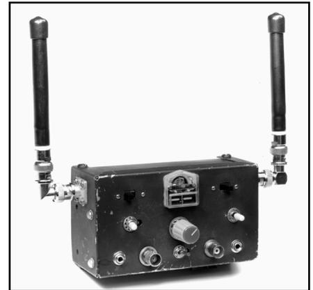
**Fig 13.48** — Field version of the Simple Seeker with helix antennas.
