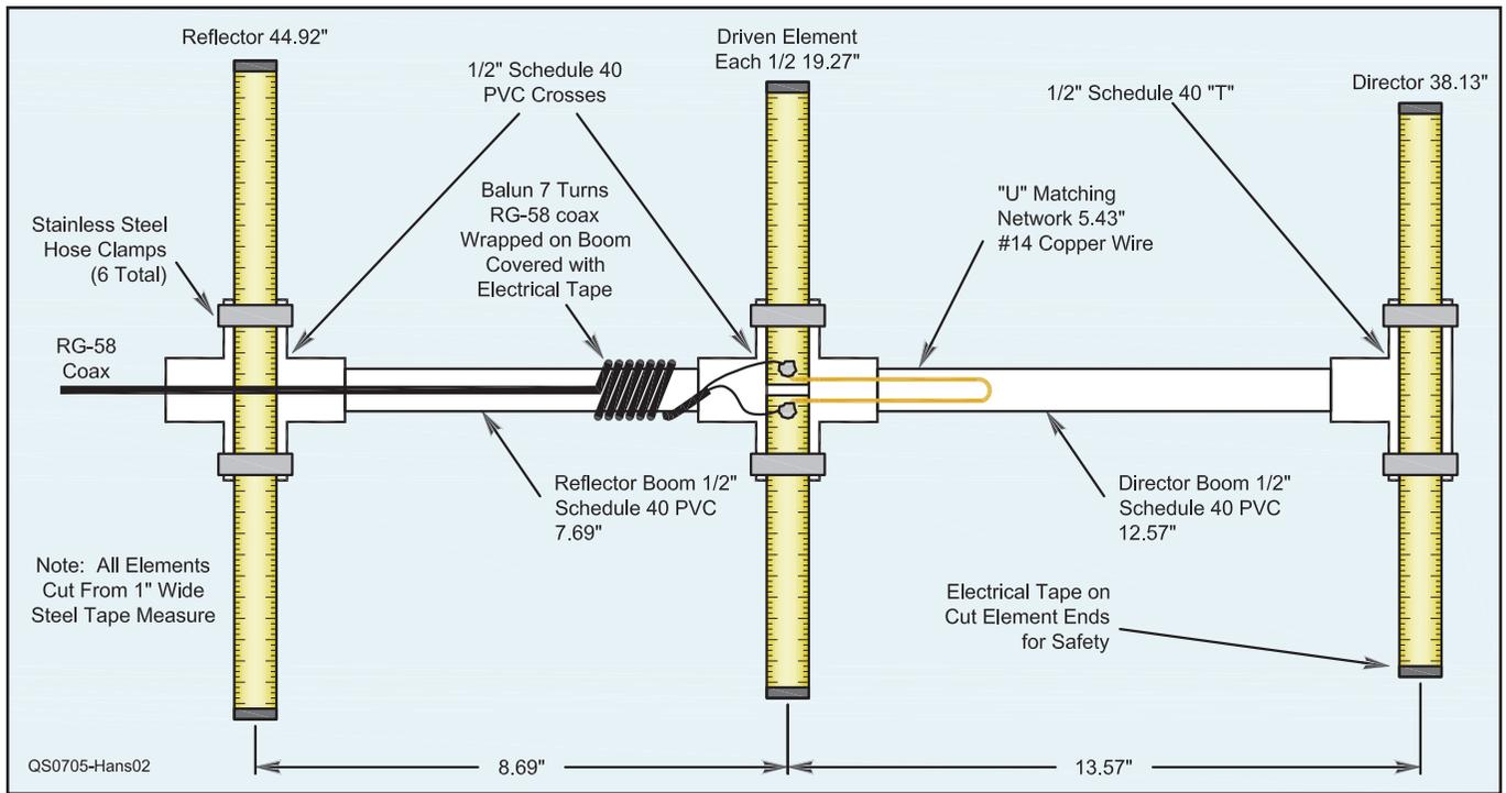
Figure 2 — 135 MHz tape measure beam assembly.
