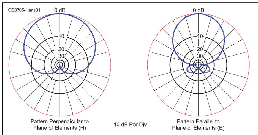
Figure 1 — YAGI-CAD predicted tape measure beam patterns.
