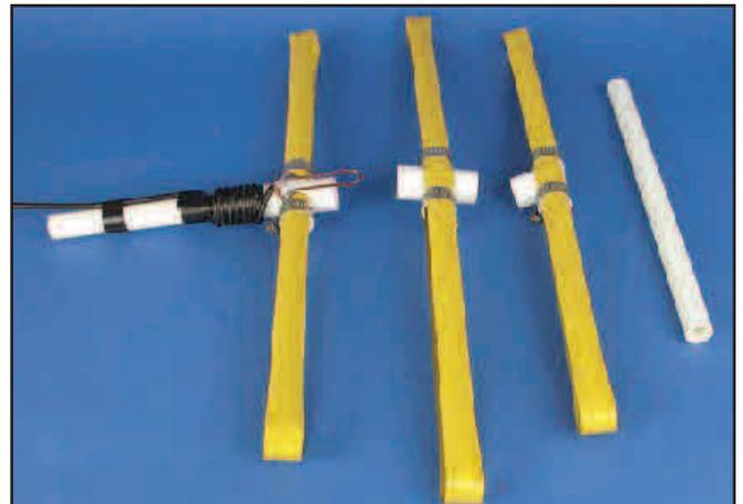
Figure 5 — Disassembled beam ready for transport.
