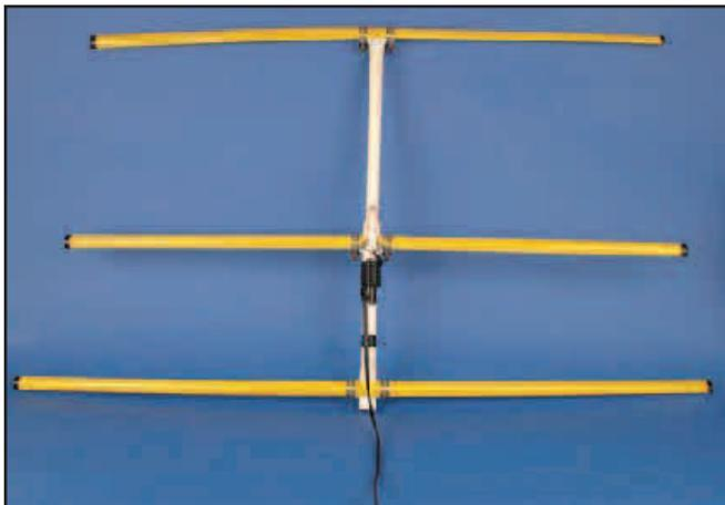
Figure 4 — Assembled 135 MHz tape measure beam.
