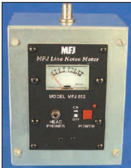
Figure 6 — Shielded MFJ-852 mounted in metal Bud box.
