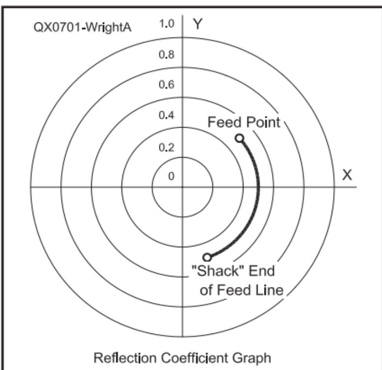
**Fig A—Plot of polar reflection coefficient. Circles represent contours of constant  $\rho$ . The starting “feed point” value, 0.5 at  $+45^\circ$ , represents an antenna impedance of  $69.1 + j 65.1 \Omega$  with  $Z_0 = 50 \Omega$ . The arc represents a 15-ft section of 50- $\Omega$ , VF 0.66 transmission line at 7 MHz, yielding a shack  $\rho$  of 0.5 at  $-71.3^\circ$ . The shack  $z$  is calculated as  $40.3 - j 50.9 \Omega$ .**
