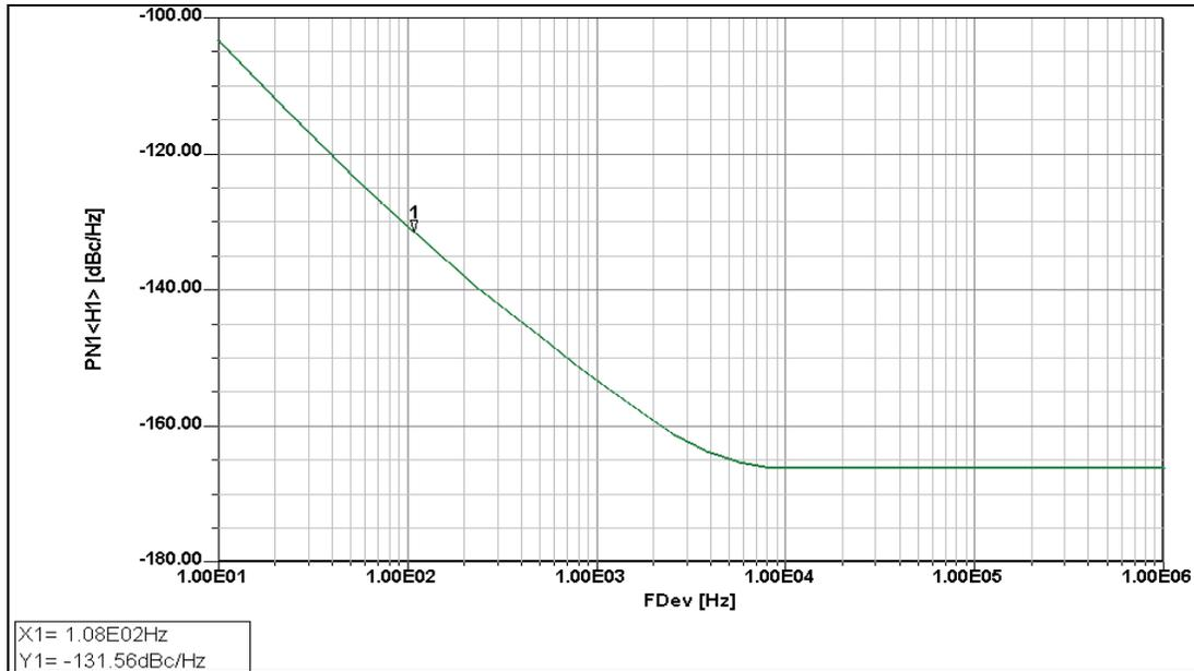
Figure 21: Simulated phase noise plot of 100MHz VCXO
