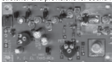
TXA5-RCb board, 1.8 x 3.5", ≥1Watt, Video only, Sound added with FMA5 board-see pg 2
