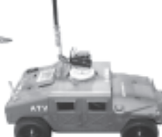
R/C Humvee by N8QPJ. Has pan & tilt camera on top.
