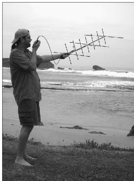
Fig 1.23 — Hams can use simple antennas and hand-held radios to contact amateur satellites, even the International Space Station. Sean Kutzko, KX9X took his satellite gear along during a vacation to Puerto Rico, making contacts via the AO-27 orbiting “bird.” [Ward Silver, (N0AX, photo)]
