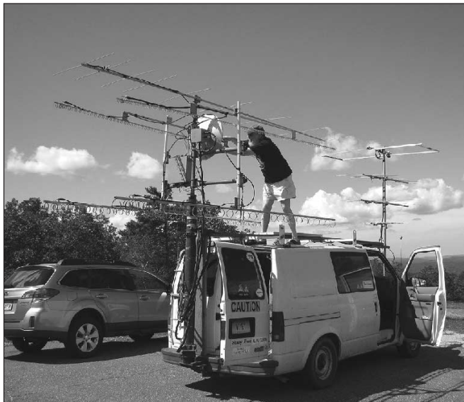
Fig 1.27 — Since antennas for the VHF, UHF and microwave bands are small enough for travel, “rover” stations are popular in competitions for these bands. Here, John D’Ausilio, W1RT adjusts his rover’s antennas during the ARRL September VHF QSO Party. [Andy Zwirko, K1RA, photo]
