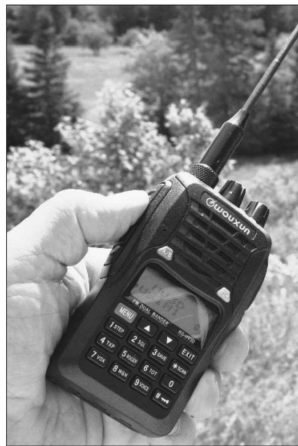
Fig 1.15 — Many thrifty hams carry a radio with them in the form of relatively inexpensive handheld transceivers such as this one, which feature long battery life and require no antenna beyond the one attached to the radio itself. Made in China, this unit cost slightly more than $100. [Rick Lindquist, WW1ME, photo]
