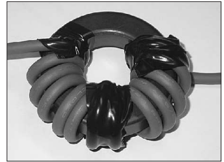
Fig 5.50 — A ferrite choke consisting of multiple turns of cable wound on a 2.4-in. OD x 1.4-in. ID x 0.5-in. toroid core.
