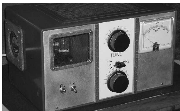
Fig 17.53 — The front panel of the Everham's Amplifier. This version is designed to cover three bands (80, 40, and 20 meters). A window is included at left to allow viewing of the tube.
