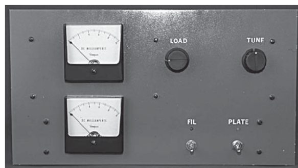
Fig 17.61 — Photo of the front panel of the 6 meter 4CX1600B amplifier.
