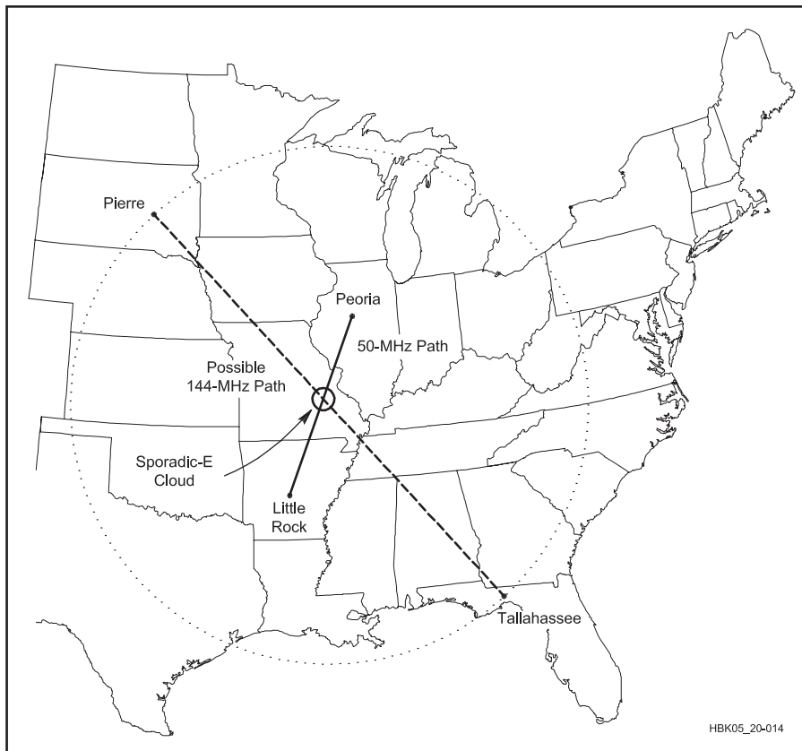
Fig 19.14 — 50 MHz sporadic E contacts of 700 km (435 miles) or shorter (such as between Peoria and Little Rock) indicate that the MUF on longer paths is above 144 MHz. Using the same sporadic E region reflecting point, 144 MHz contacts of 2200 km (1400 miles), such as between Pierre and Tallahassee, should be possible.
