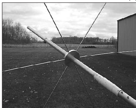
Fig 21.48 — The completed capacitance hat assembly is shown at A, and B shows a view of the upper mast assembly with the loading coil and capacitance hat.
