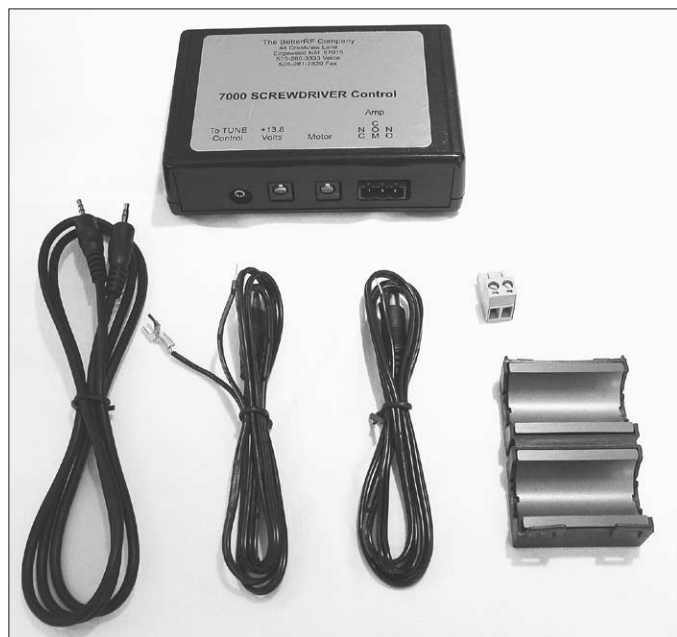
Fig 21.88 — A screwdriver antenna controller made to work with the IC-7000 transceiver.
