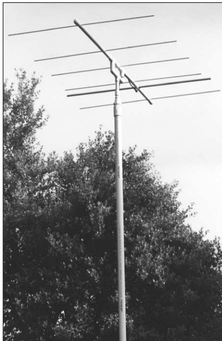
Fig 21.105 — The completed 2 meter Yagi is shown with the PVC boom and mast mount.
