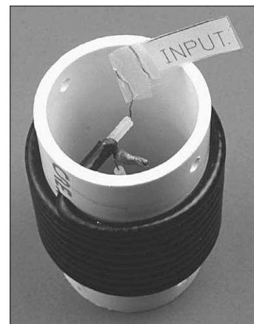
Fig 21.38 — Other views of a W8NX coax-cable trap.
