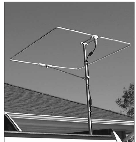
Fig 21.94 — The squalo (square halo) is a popular horizontally polarized VHF/UHF mobile antenna. The antenna shown here is made by M 2 Antenna Systems ( www.m2inc.com ).
