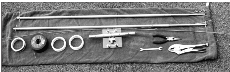
Fig 21.31 — The entire inverted-U antenna parts collection in semi-nested form, with its carrying bag. The tools stored with the antenna include a wrench to tighten the U-bolts for the mast-to-plate mount and a pair of pliers to help remove end wires from the tubing.
