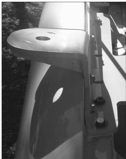
Fig 21.91 — The KE5DKM bracket mounts under the hood of a motor home.
