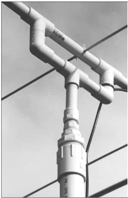
Fig 21.105 — The completed 2 meter Yagi is shown with the PVC boom and mast mount.
