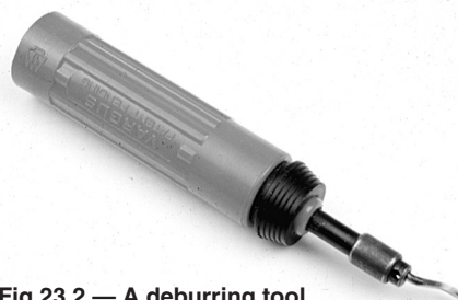
Fig 23.2 — A deburring tool is used to remove the burrs left after drilling a hole.
