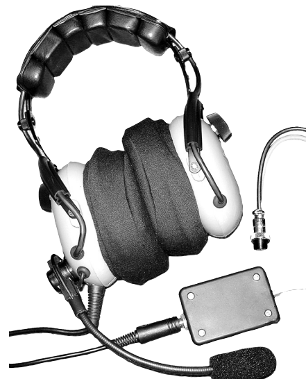
Fig 24.56 — A completed K0IZ headset/adapter. The black box contains the adapter circuit for the aviation headset.
