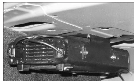
Fig 29.19 — The main body of the radio may be mounted in the vehicle's trunk or other out-of-the-way spot. Allow for plenty of ventilation.
