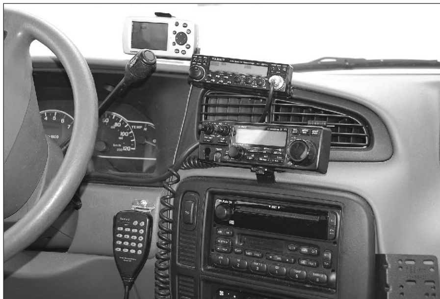
Fig 29.19 — The main body of the radio may be mounted in the vehicle's trunk or other out-of-the-way spot. Allow for plenty of ventilation.
