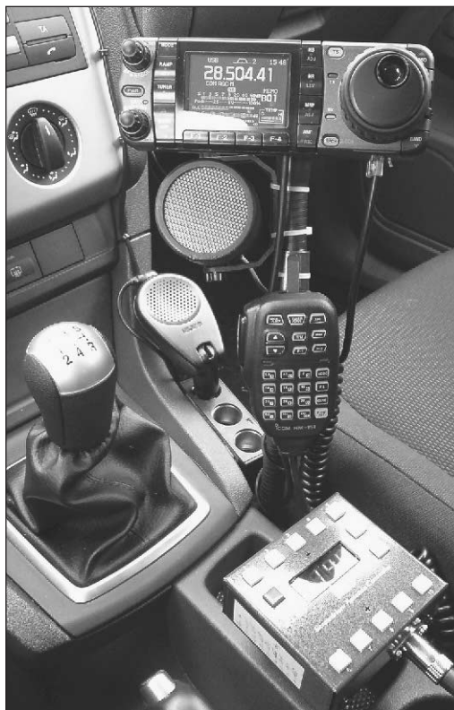
Fig 29.18 — At A, the transceiver control head is attached to one of many available mounts designed for this purpose. Mounts are typically highly adjustable, allowing the control head or radio to be positioned close to the operator. An antenna controller is mounted below the microphone. At B, HF and VHF transceiver control heads and the microphone are all mounted to the dashboard, within easy reach.
