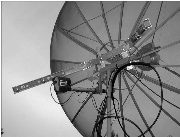
Fig 71 — Mounting arrangement, counterweights and az/el control system for the VA7MM 3 m dish.
