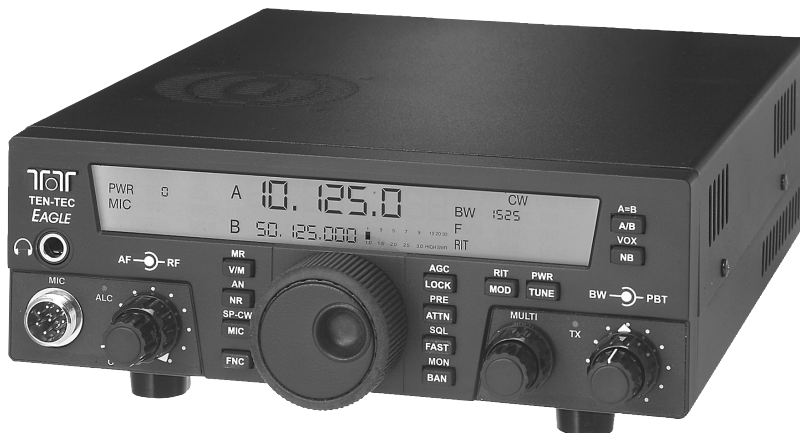
Fig 12 — The TEN-TEC Eagle, a compact HF and 6 meter transceiver provides excellent receive performance on all amateur bands.
