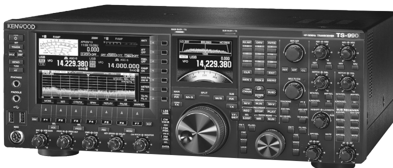
Fig 21 — The TS-990S is Kenwood's entry into the top-drawer category. It offers two receivers with high dynamic range, a 200 W transmitter and a host of interesting features.
