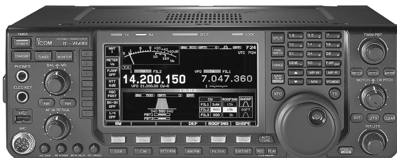
Fig 18 — The ICOM IC-7600 transceiver provides improved receiver performance through included 3, 6 and 15 kHz roofing filters.
