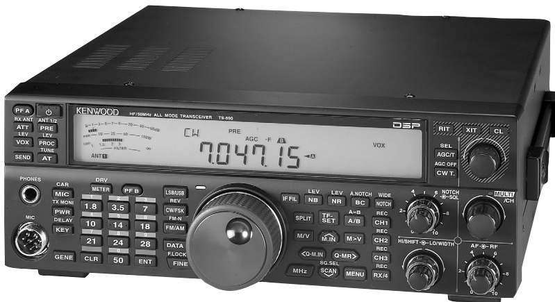
Fig 10 — The Kenwood TS-590S offers a high performance receiver on the primary HF amateur bands and many digital features.
