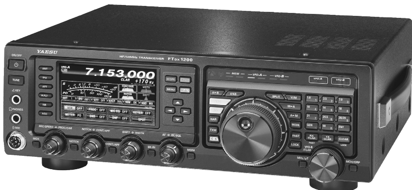
Fig 13 — The Yaesu FTDX1200 covers 160 through 6 meters and offers a colorful screen and spectrum display.
