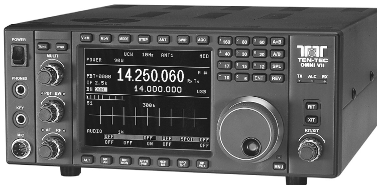
Fig 14 — The TEN-TEC Omni VII offers very good receiver performance and a single-pass panadapter.
