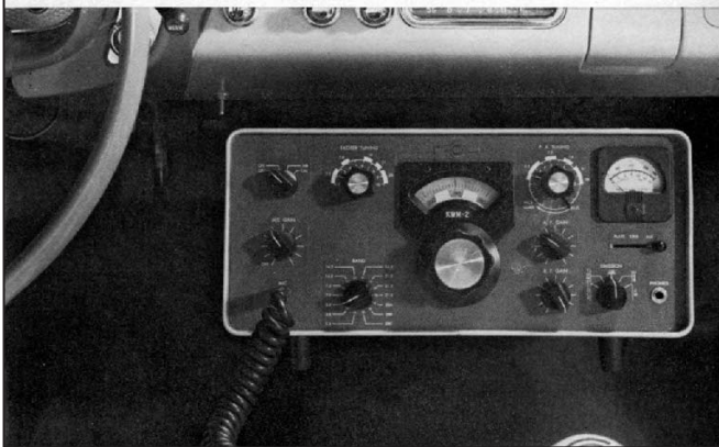
Figure 1960-5 — This Collins Radio ad featuring their KWM-2 SSB transceiver was at the leading edge of Amateur Radio technology. The architecture closely followed that of the 75A-1 receiver shown in Figure 1950-10.
