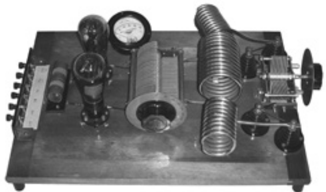
Figure 9 — Photo of a transmitter built from the schematic in Figure 8.
