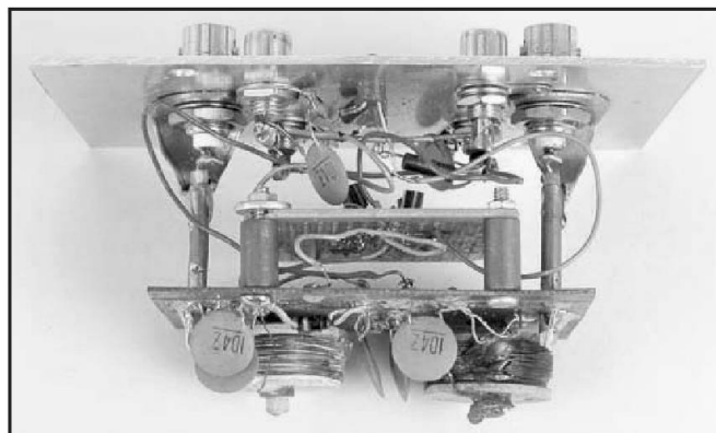
Figure 6 —Another view inside the PIN switch. The control circuitry is on a RadioShack project board secured under the diode board. Short lengths of 0.141 inch 50 Ω semi-rigid coax connect the BNC jacks to the diode board and provide mechanical support.
