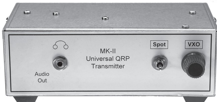
Fig 13.44 — The MKII QRP transmitter includes VXO frequency control, TR switching and a sidetone generator.
