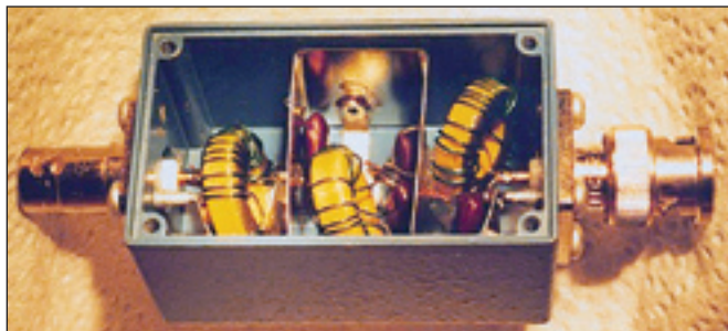
Figure 13 — 40 meter band low pass filter.
