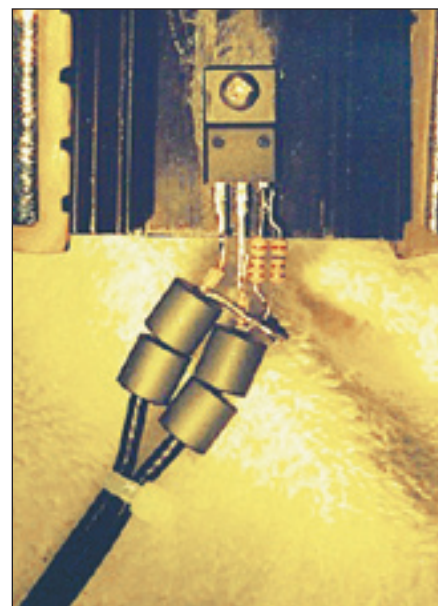
Figure 9 — Bipolar transistor with sleeve baluns.
