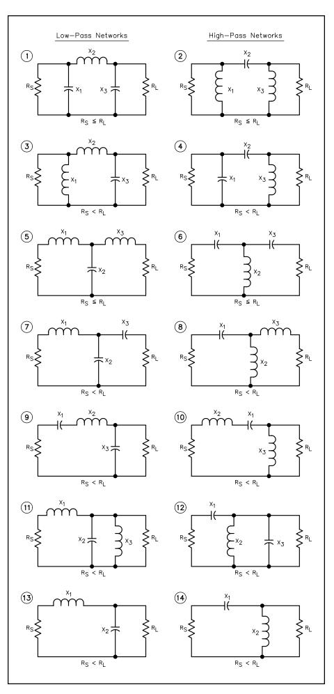
This page accompanies the ARRL Handbook software package that is available on the Handbook CD. This figure shows the 14 possible network configurations used by MATCH.EXE. Refer to this figure and enter the desired network by number when you run the program. Note that low-pass networks have an odd identifying number while high-pass networks have an even identifying number. See the Broadband Transformers file on the Handbook CD-ROM.
