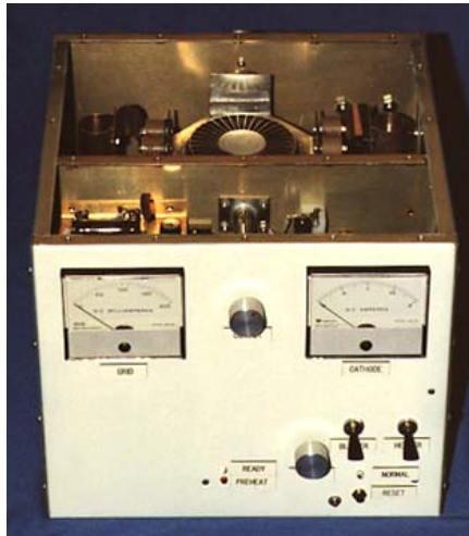
Fig 18.39—This table-top 2-meter power amplifier uses a quick-warm-up tube, a real plus when the band suddenly opens for DX and you want to join in.
