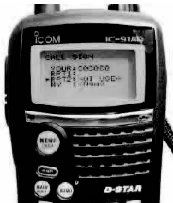
Figure 4 — Part of the extensive menu system on the IC-91AD handheld. It takes a minute to get used to what YOUR call sign and MY call sign mean. To talk to anyone, you program CQ0000 in the YOUR field. If you wanted to talk to a specific station, you'd program that station's call sign in the YOUR field. If you want to use specific linked repeaters, you use the RPT1 and RPT2 fields. This is one radio you can't operate without some quality time in the manual.
