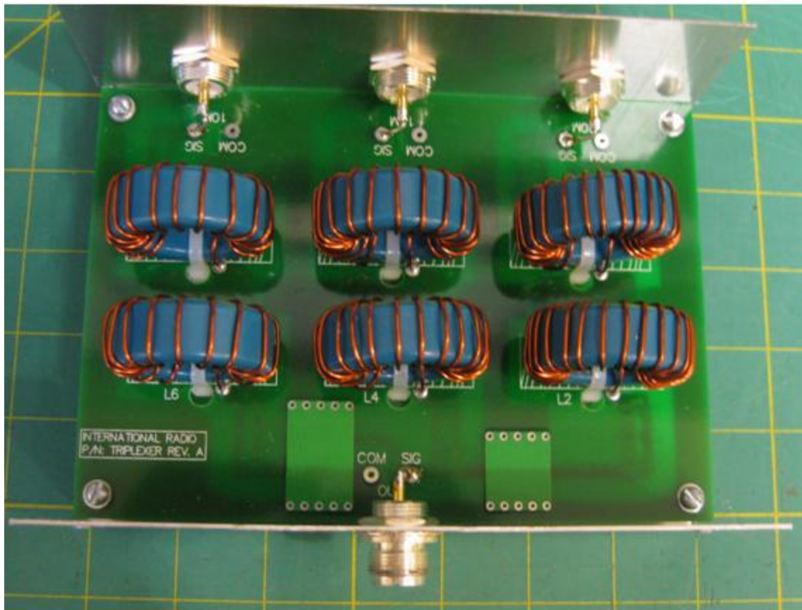
Figure 2 — The inside of the commercial production triplexer.
