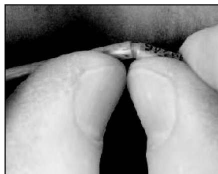
Figure 3 — Flex the cable with thumbs until the outer tubing snaps at the score line.
