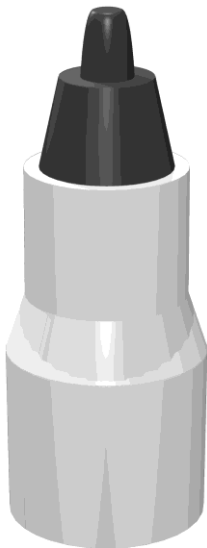
Figure 3 — Make a permanent marker into a specialized PC-board drawing tool. Simply press the marker point into a drilled hole to form a modified point as shown. More pressure produces a wider shoulder that makes larger pads on the PC board.
