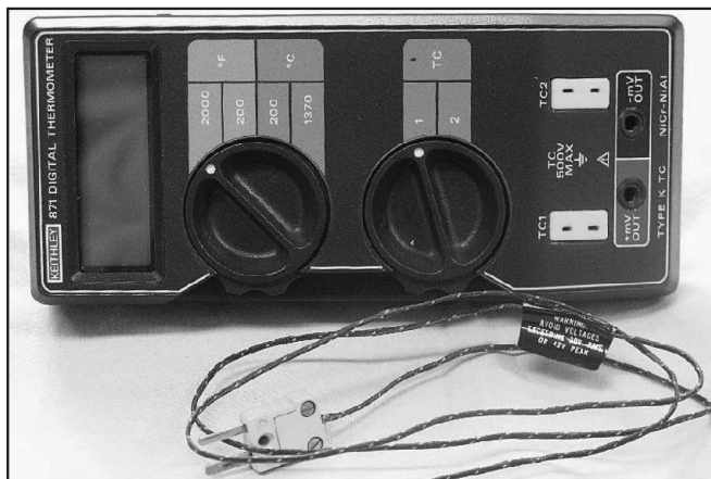
Figure 3 — Keithley electronic thermometer with type-K thermocouple probe.
