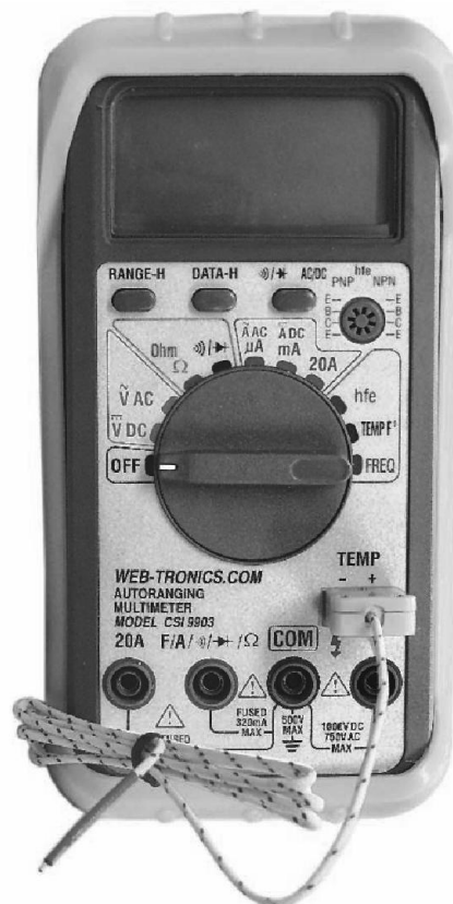
Figure 2 — Inexpensive multimeter with type-K thermocouple probe.
