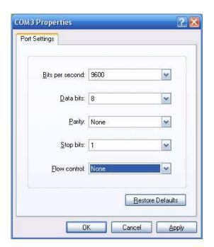
4. Now you're done. You should be able to communicate with your ID-O-Matic. If you can't, check to make sure you have the right COM port selected. Also make sure you are using a 9-pin straight through cable, NOT a null modem cable. The null modem cable has several pairs of wires crossed, and is designed to connect two computers together or a computer and a serial printer. Unfortunately there is no way to tell one from the other, except with an Ohm meter or continuity tester.
