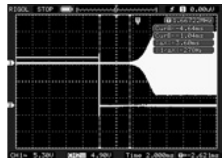
Fig 24.69 — The relay-close-to-RF timing for an ICOM IC-7200. RF output appears 3.6 ms after the amplifier relay contacts close. The relay-to-RF time can be increased 1.5-2.0 ms by substituting a small switching transistor for the relay.
