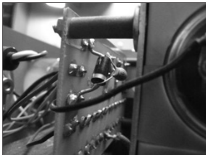
Photo A — The location of the new 1N5408 and 0.1 \mu F capacitor.
