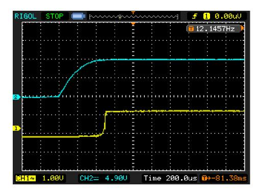
Input reed relay from transmit to receive, ~500 us to open, (200 us per division).
