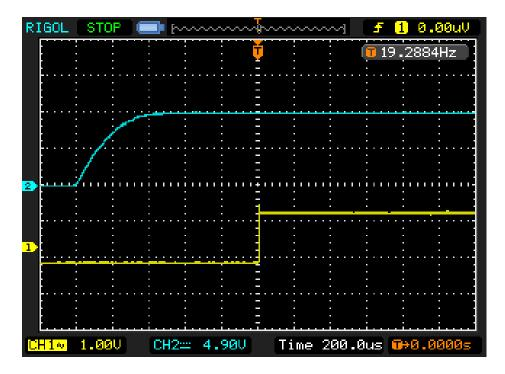
Jennings RJ1A-26N969 transitioning from transmit to receive, ~1ms to open (200 us per division).
