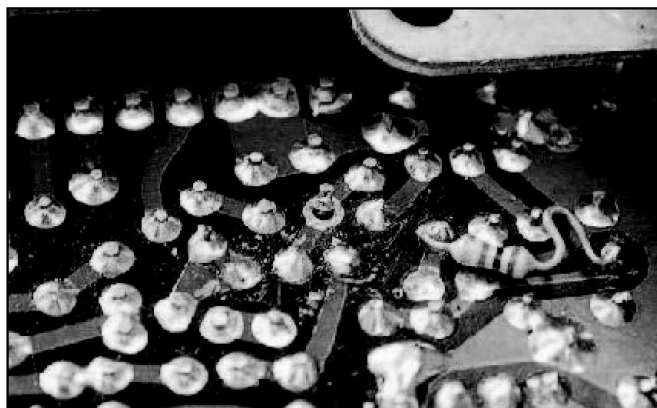
Figure 5 — Note the witch's hat fracture in the center of the photo. The lead coming from the component side of the board has a circumferential fracture and separation of the solder fillet. I have seen these many times. They are usually not as obvious. There are three others in this photo. Hint — look up.
