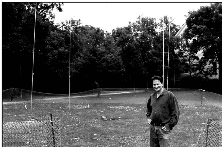
Figure 3—Karl, AA9MN, designer of the NSRC 4-square antenna, standing in front of it. The area in which MPE limits can be exceeded has been made inaccessible by orange plastic safety fencing.
