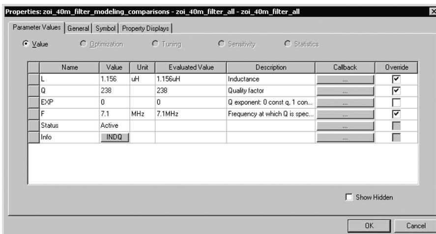
Fig 6.26 — Properties dialog for the *Ansoft Designer SV 2* INDQ component, showing settings for *Q*.
