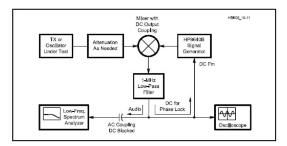
Figure 3 — Arrangement for measuring phase noise by directly converting the signal under test to audio. The spectrum analyzer views the signal's noise sidebands as audio; the signal's carrier, converted to dc, provides a feedback signal to phase-lock the Hewlett-Packard HP8640B signal generator to the signal under test.
