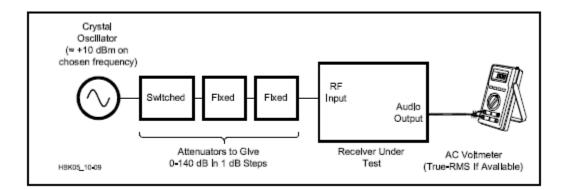
Figure 1 — Setup for measuring receiver-oscillator phase noise.
