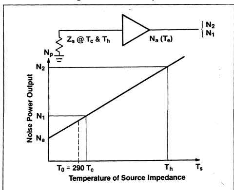
The Noise Figure Measurement by the Y-Factor Method
