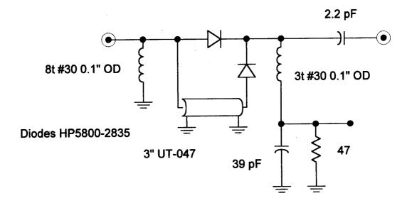
Not only does addition of the bias resistor permit optimizing the doubler for much higher drive levels, the bias circuit provides a built-in test point that provides a calibrated output reading. Two different doublers, one using a T4:1 transformer and the other using a half-wave UT-085 balun were measured, using a 47 ohm bias resistor. The voltage across the bias resistor versus the second harmonic (desired) output level are shown in the figure 5 plot below.
