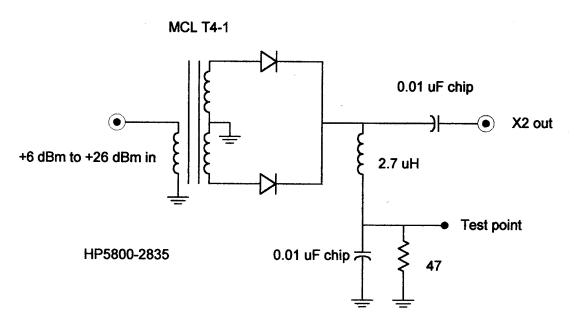
A more general form of doubler is shown in figure 2, which includes a low-pass filter on the input. Balanced doublers require sine wave drive. The presence of even small amounts of even or odd harmonics will dramatically reduce the desired output and increase the undesired outputs. Square wave drive to the circuit in figure 1 (no odd harmonics, 3rd harmonic 9.5 dB down, 5th harmonic 14 dB down, 7th harmonic 17 dB
