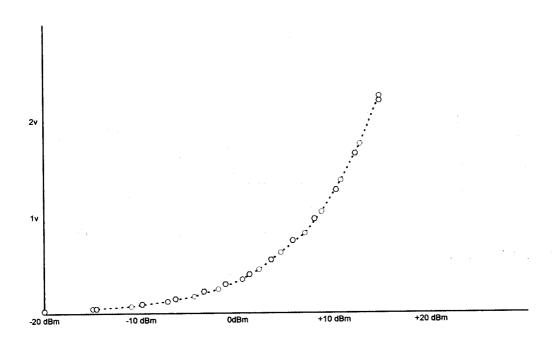
The open circles are from the T4-1 transformer doubler and the filled circles are from the UT-085 balun doubler. Clearly the DC voltage across the 47 ohm bias resistor provides a useful measurement of output power. There is a relationship between bias voltage and frequency doubler output power, which can be used as a power indicator, but this voltage will likely change when the doubler drives something other than a perfect 50 ohm RF load.
