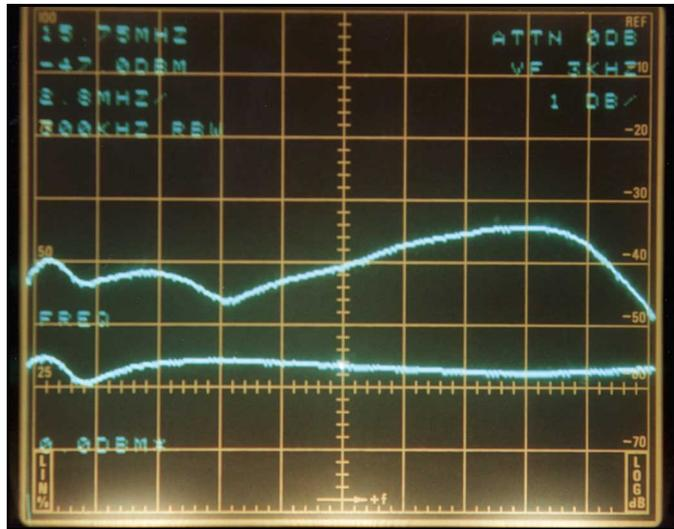
**Fig 6—Gain variation, 1.8 MHz to 29.7 MHz, 1.0 dB per division vertical scale—The lower trace is a reference sweep that bypasses the 100-W amplifier—The response bump at low frequency is an artifact of the tracking generator.**
