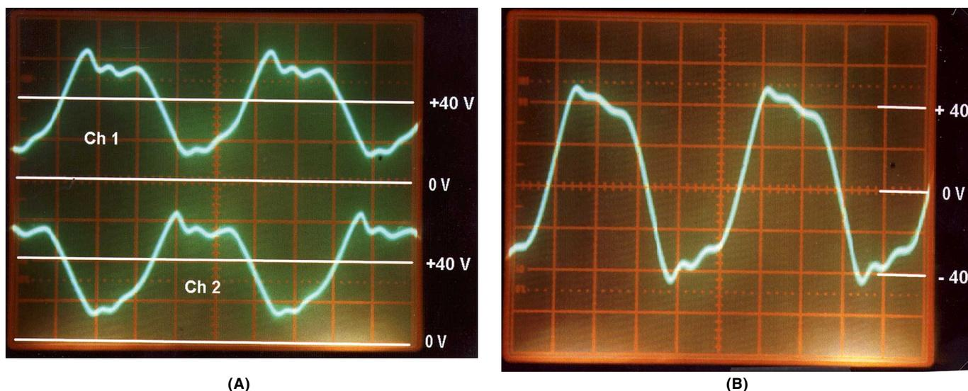
Fig 7—(A) drain and (B) drain-to-drain oscilloscope waveforms.
