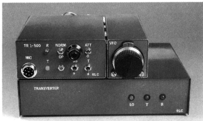
Fig 3—The first no-tune, single-conversion 1296-MHz transceiver that follows the block diagram of Fig 2.
