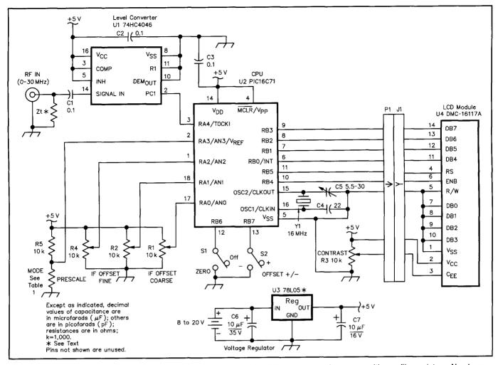
Figure 1—Schematic of the DFD. Unless otherwise specified, use 1/4-W, 5%-tolerance carbon-composition or film resistors. Numbers in parentheses are Digi-Key stock numbers. (All parts are available from Almost All Digital Electronics.)¹ Equivalent parts may be substituted for those shown.
