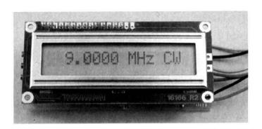
Build this inexpensive, miniature counter for your test bench or as a display for your superhet or direct-conversion HF, VHF, UHF or SHF rig. Adjustable IF offset and prescale compensation make its application to your radio a snap!
