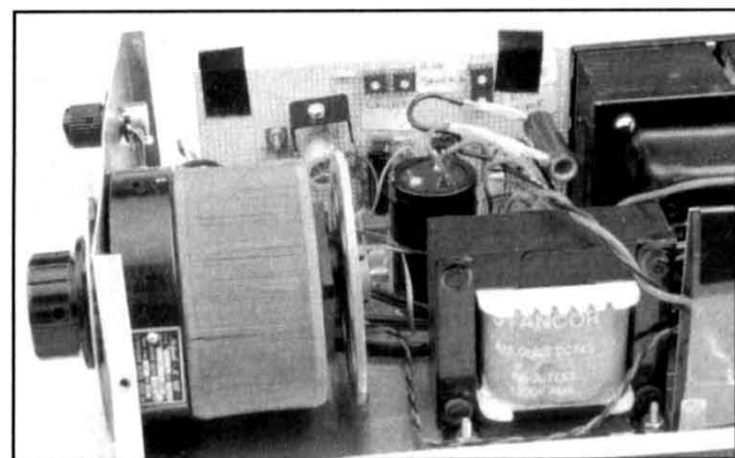
Figure 12—The keyed power supply with the cover removed, viewed from the side. T1 is mounted on the back plate, along with the fuse and connectors for the dc output, a keying line to the NorCal 40A and the ac line input. The TUNE switch keys the amplifier for testing. The variable autotransformer is on the left, mounted to the front panel. In the center foreground, mounted to the base plate, is L1, the 25-mH choke. Mylar sheets are taped to the perfboards for electrical isolation. The large components are attached directly to the box. The IRFP340 is mounted on the bottom of the box using a Berquist K10-104 Kapton insulating pad, #6-32 screw and a torque of 10 inch-pounds. The other shaping circuit components are mounted on perfboard. Layout is not critical.
