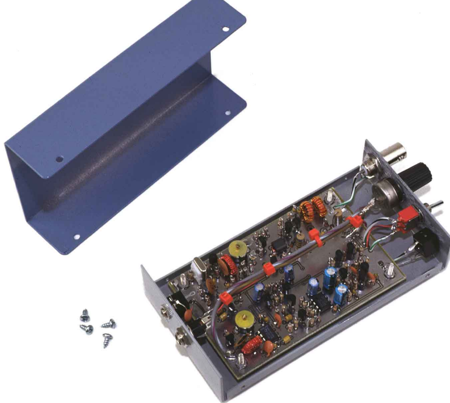
This Micromountaineer is housed in an LMB enclosure. Take care to remove paint on the inside of these enclosures to ensure contact with grounded components.
