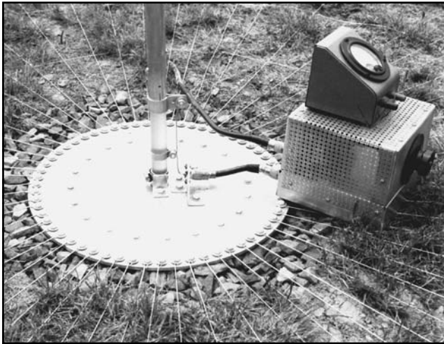
Fig 67— Base of the vertical antenna showing the 60 radial wires. The aluminum disc is 15 inches in diameter and \frac{1}{4} inches thick. Sixty tapped holes for \frac{1}{4} -20 aluminum hex-head bolts form the outer ring and 20 form the inner ring. The inner bolts were used for performance comparisons with more than 60 radials. The insulator is polystyrene material (phenolic or Plexiglas suitable) with a 1-inch diameter. Also shown is the impedance bridge used for measuring input resistance.
