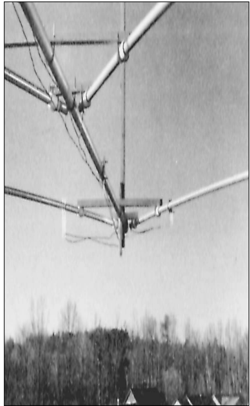
Fig 30 —The feed arrangement, using a right-angle chassis-mounted BNC connector, modified by removing a portion of the flange. A short length of bus wire connects the center pin to the opposite feeder conductor.
