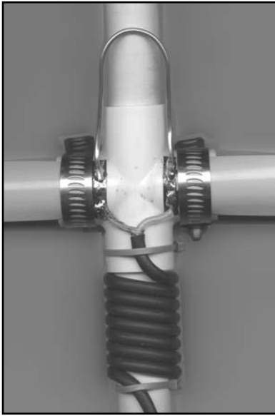
Fig 45—Photo of driven-element mounted to PVC tee using hose clamps. The hairpin match wires is shown here soldered to the tape-measure elements, along with the RG-58 feed line.
