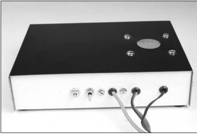
Fig 43 —The rear panel of the DF unit supports the two DPDT PHASE toggle switches. Grommets in the panel holes allow abrasion-free passage of the antenna, dc-power and audio cables. The dc power cord is outfitted with an inline fuse holder and a male Jones plug. A six-pin female Molex connector (five pins are used) feeds the four antennas. The audio-input cable is terminated in a \frac{1}{8} -inch diameter male plug.
