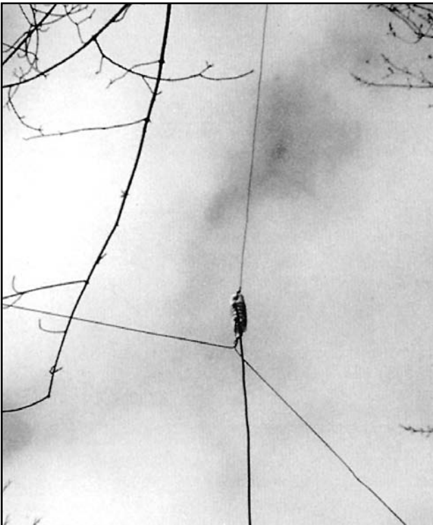
Fig 4—The feed point of the tree-mounted ground-plane antenna. The opposite ends of the two radial wires may be connected to stakes or other convenient points.
