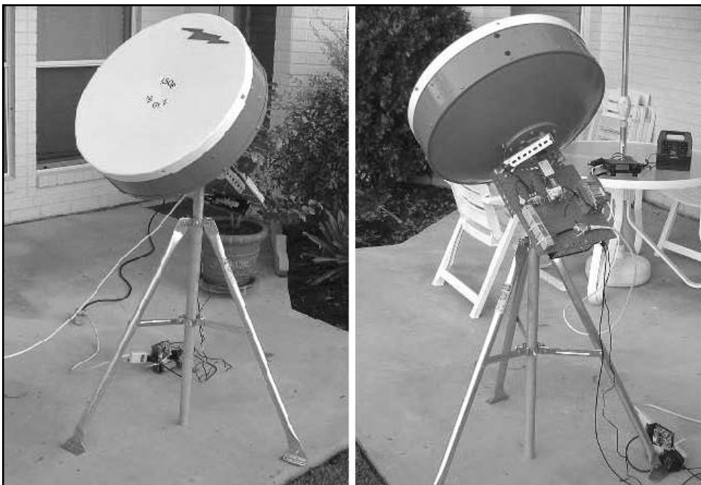
Fig 38 —K5OE found this K-band dish on the Web and has set it up for the AO-40 K-band downlink. (K5OE photo.)
