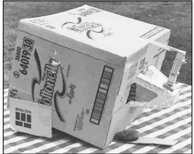
Fig 35—Side view of the downlink pyramidal horn showing the elevation control supports and how the downconverter is attached to the horn. The downconverter is pulled forward by the tape to align the probe wire parallel to the rear surface of the horn.
