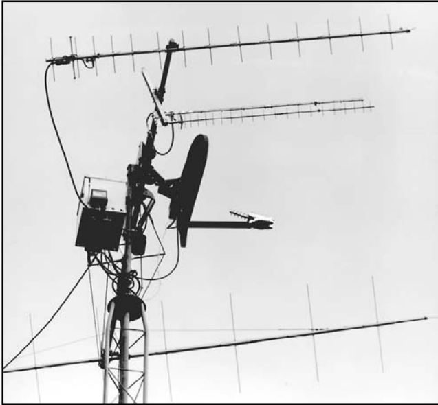
Fig 20—Details of WD4FAB’s tower cluster of satellite antennas including a home-brew elevation rotator. Top to bottom: M 2 436-CP30, a CP U-band antenna; two M 2 23CM22EZA antennas in a CP array for L band; “FABStar” dish antenna with helix feed for S band; M 2 2M-CP22, a CP V-band antenna (only partially shown.) To left of dish antenna is a NEMA4 equipment box with an internal 40-W L-band amplifier, and also hosts externally mounted preamplifiers. (WD4FAB photo)
