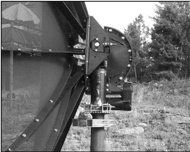
Fig 67 —A modified TVRO dish mount is shown using an Az-EI mount and a sector-gear drive for the elevation. (WØLMD photo.)
