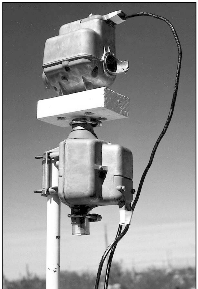
Fig 65—At left, Yaesu Az-EI antenna-rotator mounting system is shown. Note that antenna loads must be more carefully balanced on this rotator than in the previously shown systems. At right, VE5FP has a solution for his Az-EI rotators by bolting two of them together in his “An Inexpensive Az-EI Rotator System”, QST, December 1998.
