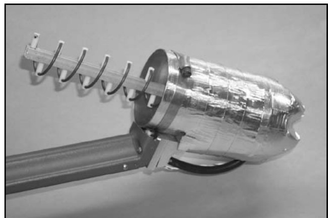
Fig 45—Rain cover for preamp using a two-liter soft-drink bottle with aluminum foil tape for protection from sun damage. (WD4FAB photo.)
