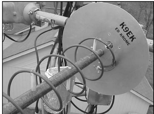
Fig 59 —At top, the method of reinforcing the reflector screen with aluminum channel stock is shown. In this version of the antenna, the three angle brackets of Fig 58 have been replaced with a surplus aluminum flange assembly. (W0CY photo.) At bottom, this helix view shows the details of a 1/4-turn matching transformer, as discussed in the text. (K9EK photo.)
