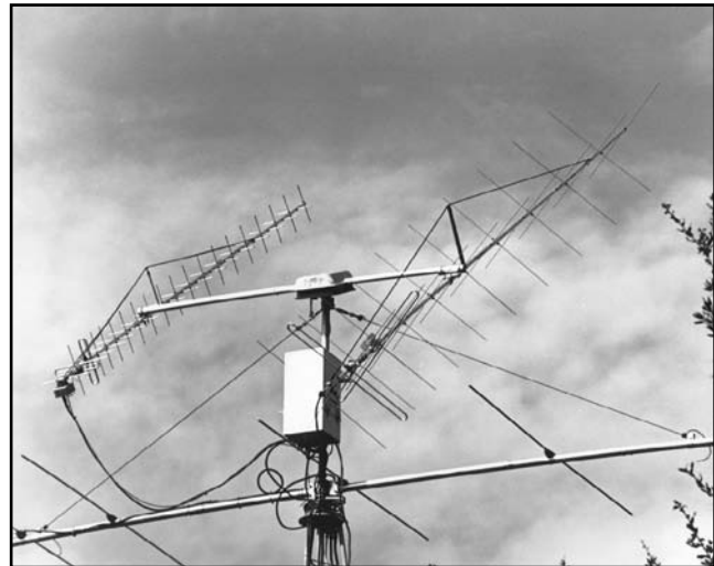
Fig 6— Dick Jansson, WD4FAB, used these 2-meter and 70-cm crossed Yagi's in RHCP for AO-10 and AO-13 operations. The satellite antennas are shown mounted above a 6-meter long-boom Yagi.
