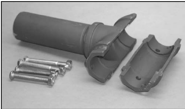
Fig 46 —Welded pipefitting mount bracket for FABStar dish antenna. (WD4FAB photo.)
