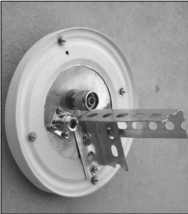
Fig 55—Rear of the completed feed. (K5OE photo; courtesy of The AMSAT Journal .)
