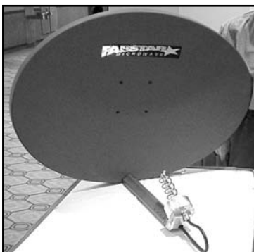
Fig 30 —PrimeStar offset-fed dish with WD4FAB's helix-feed antenna. N0NSV was so pleased with the modification that he renamed the dish "FABStar," and made a new label! (N0NSV photo.)
