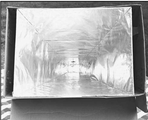
Fig 34—Front view of the downlink pyramidal horn showing how it is mounted in the support carton. Notice the coax probe at the back of the horn.
