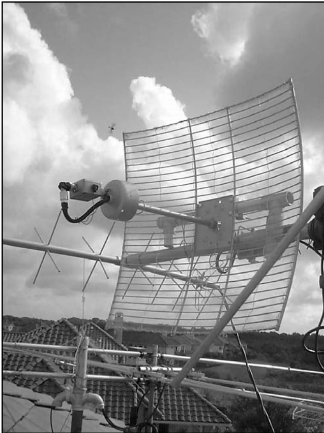
Fig 29 —Mesh modification of an MMDS dish antenna by Jerry Brown, K5OE, with a helix-CP feed and DEM preamplifier mounted directly to the helix feed point. (K5OE photo.)
