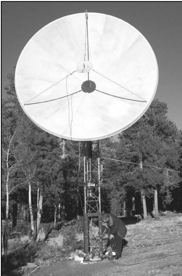
Fig 26 —WØLMD found the ultimate in this 14-foot dish for AO-40, with a tri-band patch feed and Az-El mount. ( WØLMD photo. )
