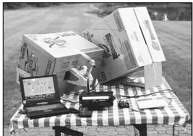
Fig 32 —A complete satellite station with the tracking laptop, FT-847 transceiver, and both downlink and uplink cardboard-box antennas.
