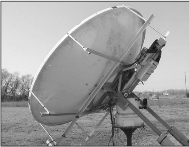
Fig 93—Strengthening struts W5LUA added to the back of his dish to hold down distortion. (Photo courtesy W5LUA.)
