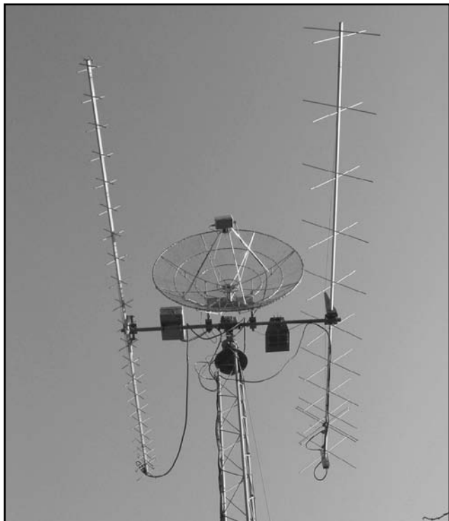
Fig 22 —Wilfred Carey, ZS6JT, constructed this cluster of satellite and EME antennas. Left to right: 2 × 23-element offset feed Yagi for U band; 1.64-meter dish with 2¼-turn helix feed for S band; 2 × 11-element coplanar feed Yagi for V band. (ZS6JT photo.)
