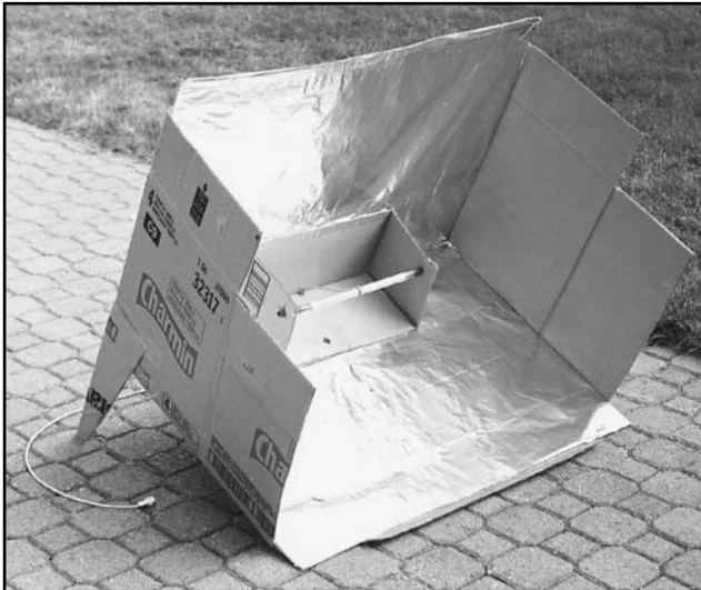
Fig 33—The completed high-performance corner-reflector uplink antenna for U band. Note how the box corners hold the reflectors and dipole feed in place. The rear legs set the antenna elevation to 20°—this gives good coverage at the design latitude but will need modification for other stations.
