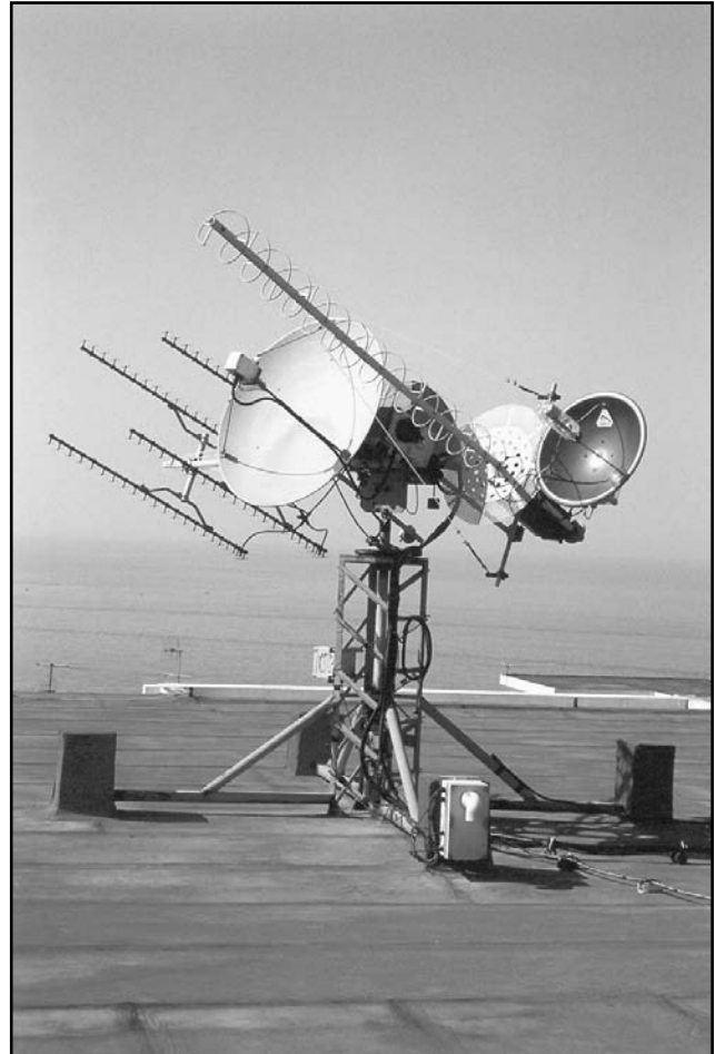
Fig 21—Domenico, I8CVS, has this cluster of satellite antennas for AO-40. Left to right: array of 4 × 23-element Yagi horizontally polarized for L band; 1.2-meter dish with 3-turn helix feed for S band; 15-turn RHCP helical antenna for U band; 60-cm dish for X band. All microwave preamplifiers and power amplifiers are homebrew and are mounted on this antenna cluster. (I8CVS photo.)
