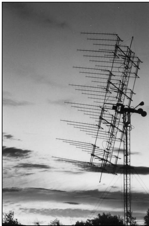
Fig 77 —NC11's magnificent 48-Yagi 70-cm EME array. (Photo courtesy NC11.)
