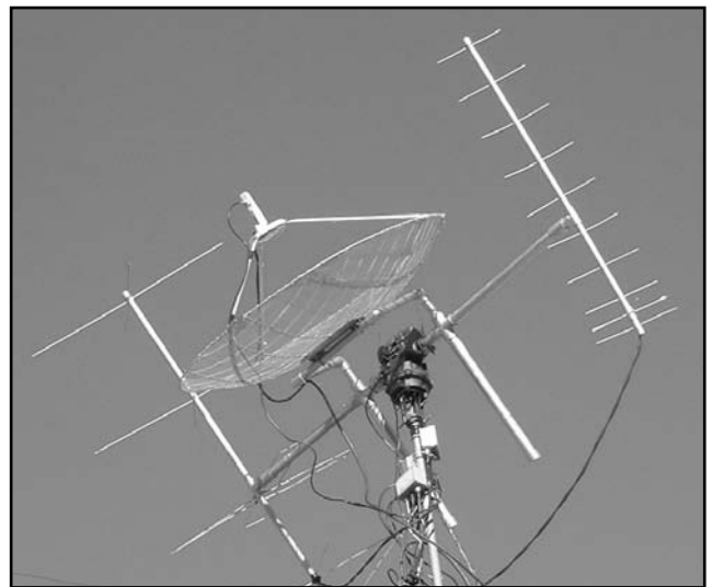
Fig 50—The 1.2-meter dish with dual-band patch feed installed. (K5OE photo; courtesy of The AMSAT Journal.)
