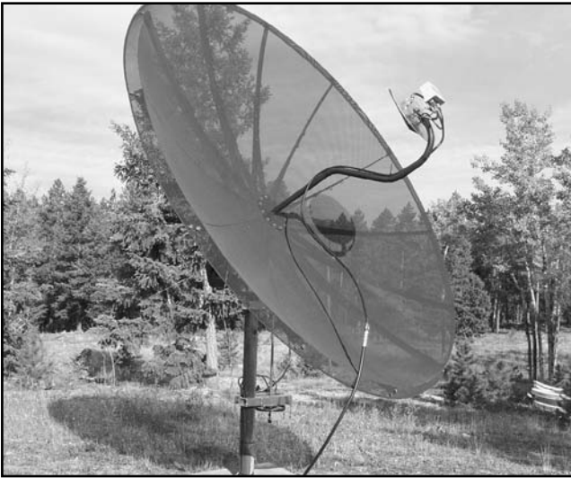
Fig 25 —WØLMD increased to this 10-foot dish for AO-40 operations, with a tri-band patch feed for U, L, and S bands on an Az-El mount. ( WØLMD photo. )
