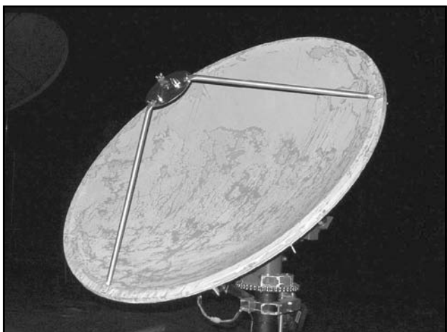
Fig 23 —Robert Suding, W0LMD, modified this 4-foot dish antenna with a patch feed for S band and an Az-EI mount. (W0LMD photo.)
