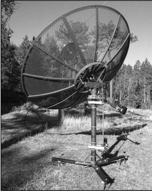
Fig 69 —A completed TVRO dish Az-El mounting system is shown, using a jackscrew elevation drive. (W0LMD photo.)
