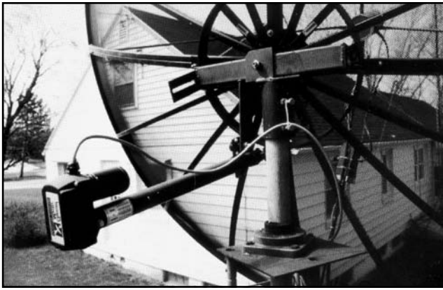
Fig 90—Elevation system, showing modified TVRO mount.
