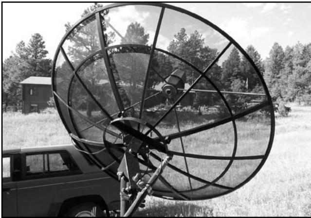
Fig 66 —A TVRO dish-drive system is shown on its polar mount, using a protected drive-screw mechanism. (WØLMD photo.)
