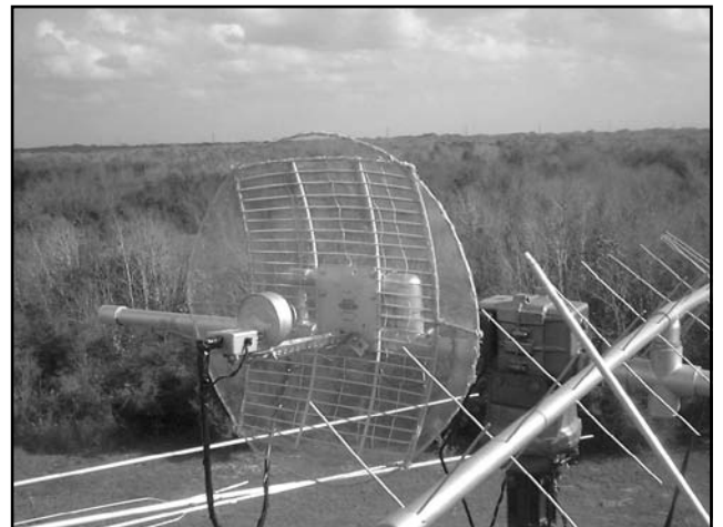
Fig 28 —K5GNA's "circularized" mesh modification of an MMDS dish antenna with a helix-CP feed and DEP preamp. The dish modification reduces the spillover loss by making the antenna fully circular. ( K5OE photo. )
